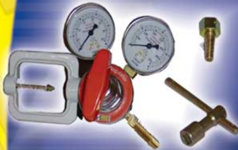
HD 103 AC Acetylene Regulator Rated Inlet Pressure: 0 – 40 kg/cm 2 Rated Outlet Pressure: 0 – 2.5 kg/cm 2 Flow: 5 m 3 /h Gauge Diameter : 60 mm Approvals: CE
