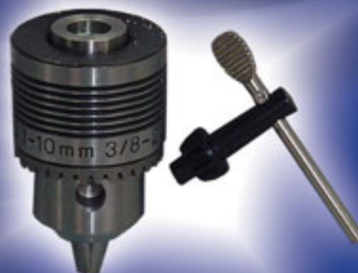
HD 710 Drill Chuck With H Type Key Professional Ball Bearing Build In DIN 6349 Type 1-10 mm 3/8" - 24 UNF CE
